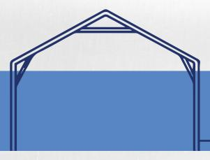
The COLD FORMED building frame consists of posts (column), rafters, knee and apex braces. The columns and rafters are straight.
